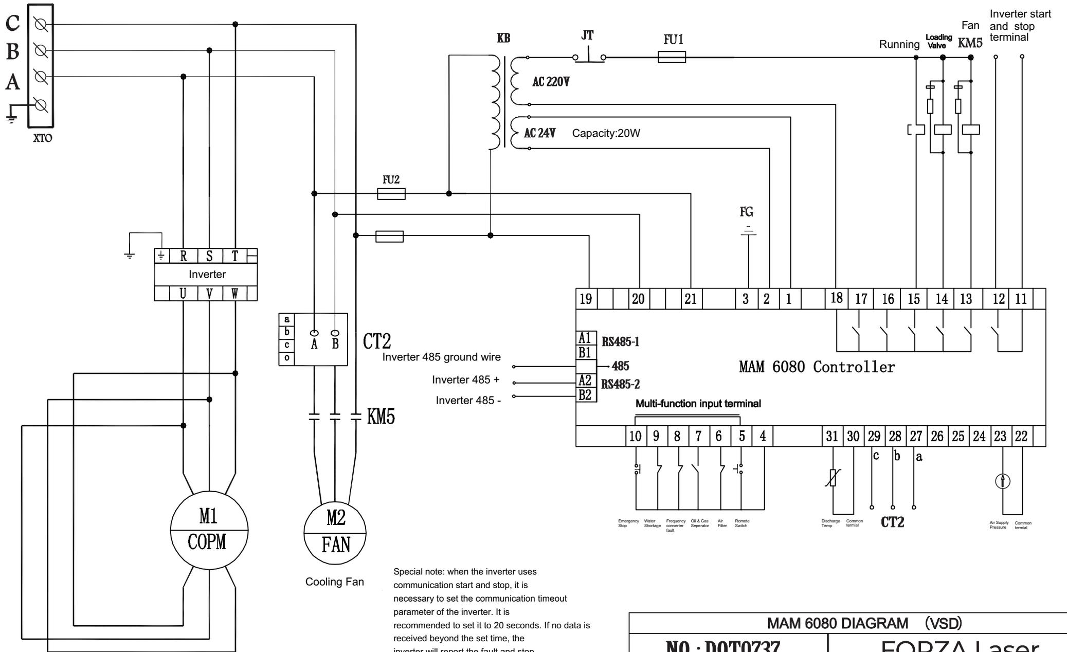
Special note: when the inverter uses communication start and stop, it is necessary to set the communication timeout parameter of the inverter. It is recommended to set it to 20 seconds. If no data is received beyond the set time, the inverter will report the fault and stop.
